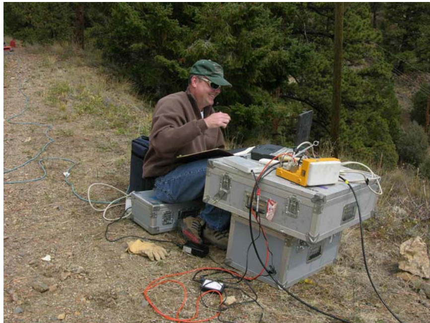
Figure 20. The operator console (laptop computer) and up hole electronics (yellow box sitting on the shipping containers) for the Mala RAMAC borehole radar.
