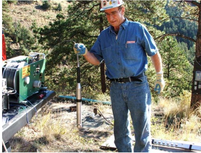
Figure 12. Sparker seismic source.
