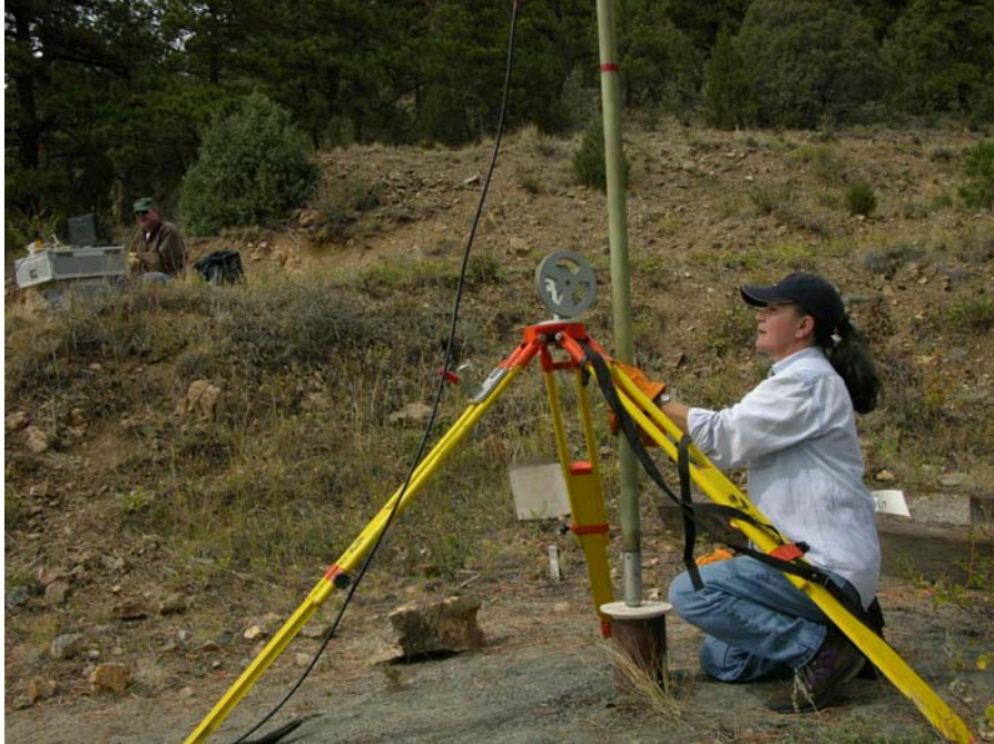
Figure 21. Holding the radar tool at top of hole for airwave transit time calibration.
