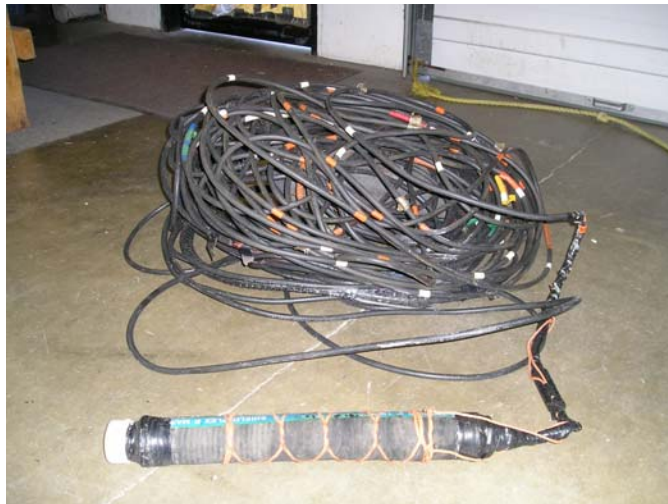
Figure 11. Etrema swept frequency seismic source.
