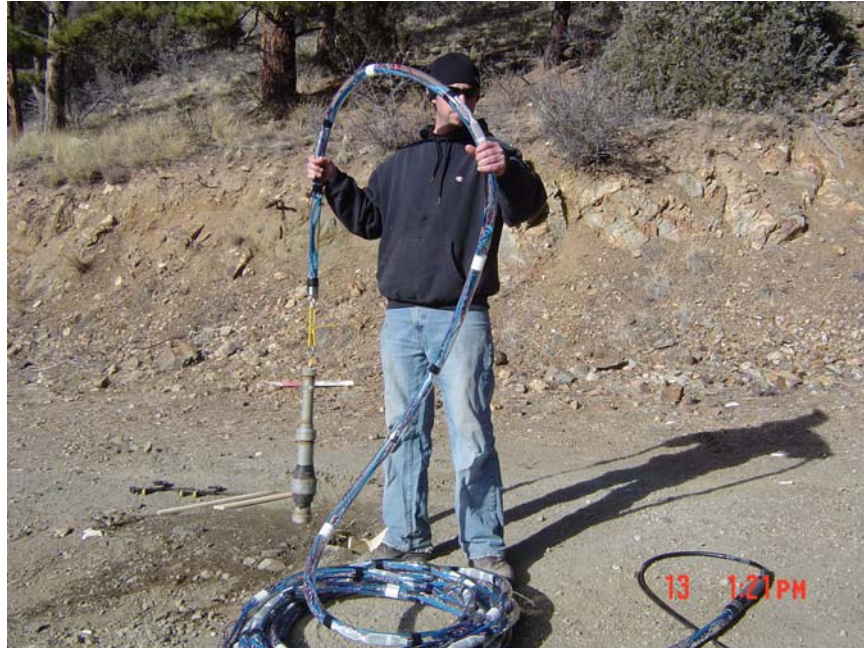
Figure 14. The 24-channel hydrophone array.
