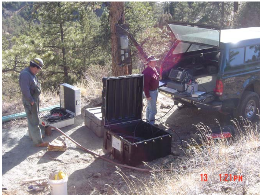
Figure 15. Data acquisition setup, with water being added to borehole U1A.
