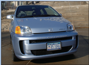
This Honda FCX fuel cell car runs on hydrogen, with water vapor its only emission.
