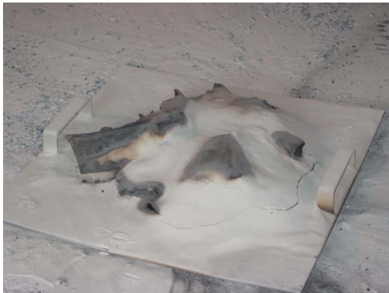
Figure 6. Sodium Chloride-Formed Hard Crust
