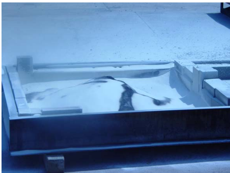
Figure 5. Fire Continuing to Burn Underneath the Dry Sodium Chloride Powder
