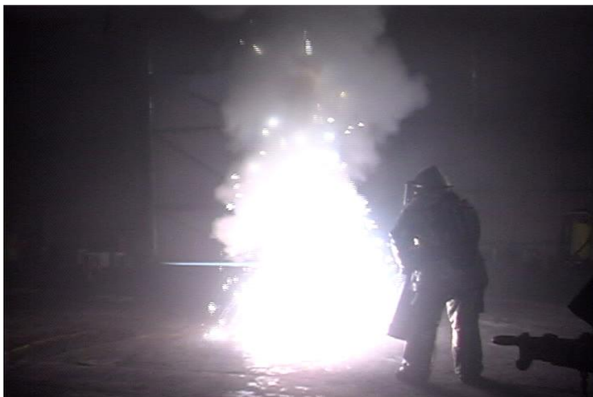
Figure 7. Magnesium Fire Flare-Up From Application of FEM-12 SC
