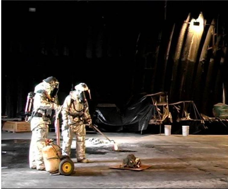
Figure 2. Fire Technicians Using Propane Torch to Ignite Magnesium
