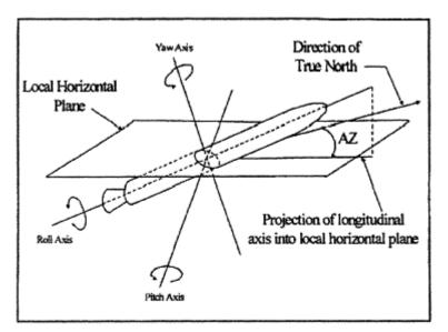
Figure A417.9-4, Hlustrative Longitudinal Axis Azimuth (AZ)
