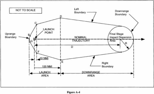
Figure A-4 Flight Corridor for Guided Sub-Orbital Launch Vehicles
