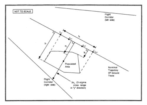
Figure C-2: Analysis of an Appendix B Flight Corridor
