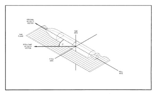
Figure B-2: Velocity Vector Turn Angle in Yaw Plane
