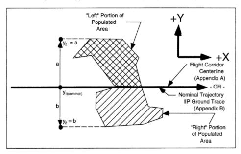
Figure C-4: Flight Azimuth Intersecting a Populated Area
