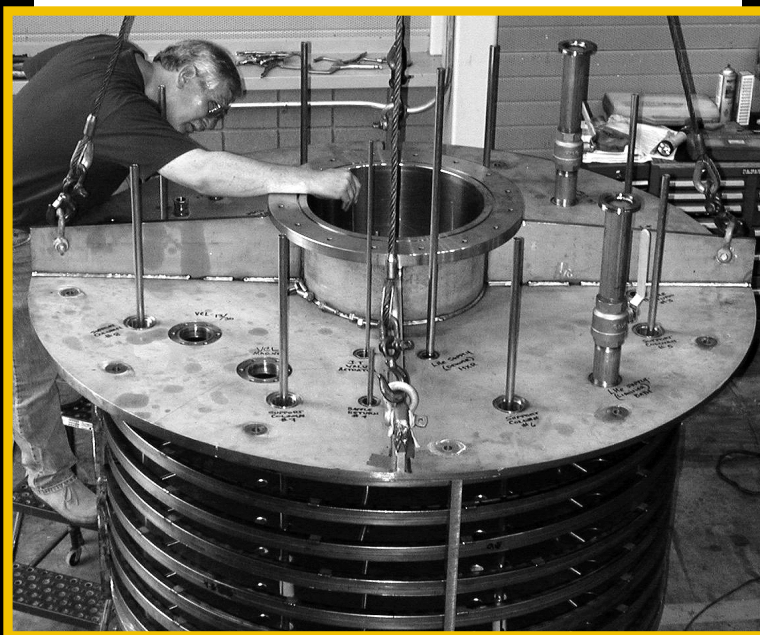
Figure 2. The bucket test baffle system is shown here undergoing its final assembly.
