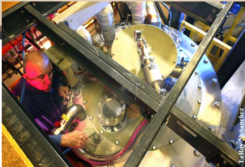
Dwight Rickel of the National High Magnetic Field Laboratory's Pulsed Field Facility at Los Alamos National checks the 100 Tesla Multi-shot Magnet. Recently commissioned for user operation at 85 tesla, the magnet opens up new frontiers for scientific research.
