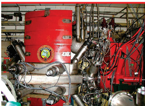
Figure 1. The Sweeper in the N4 vault at the NSCL. The quadrupole triplet is to the right and the focal plane detector is to the left. MoNA is not shown.
