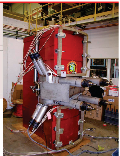
Figure 3. Test fitting the trim coils on the Sweeper before installation in the vault.
