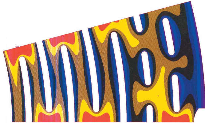
Figure 3. Mid-plane stress of the new A2 coil.
