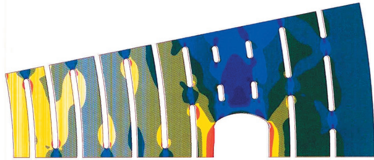
Figure 2. Mid-plane temperature of the new A2 coil.
