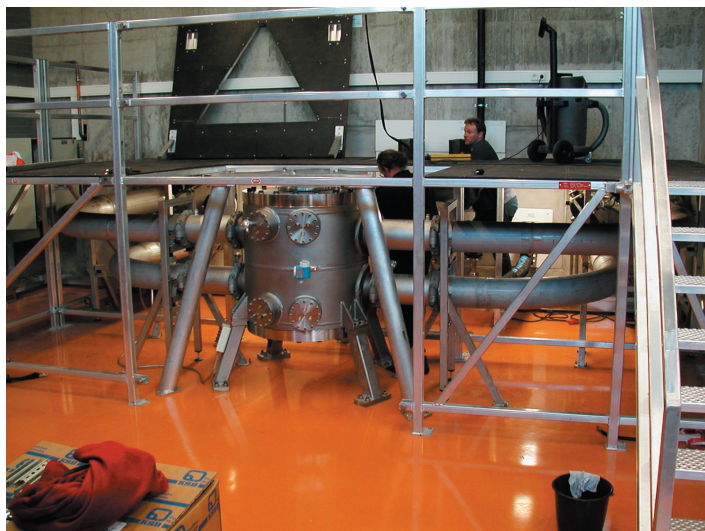
Technicians attach power cables to the 33 T magnet in Nijmegen.
