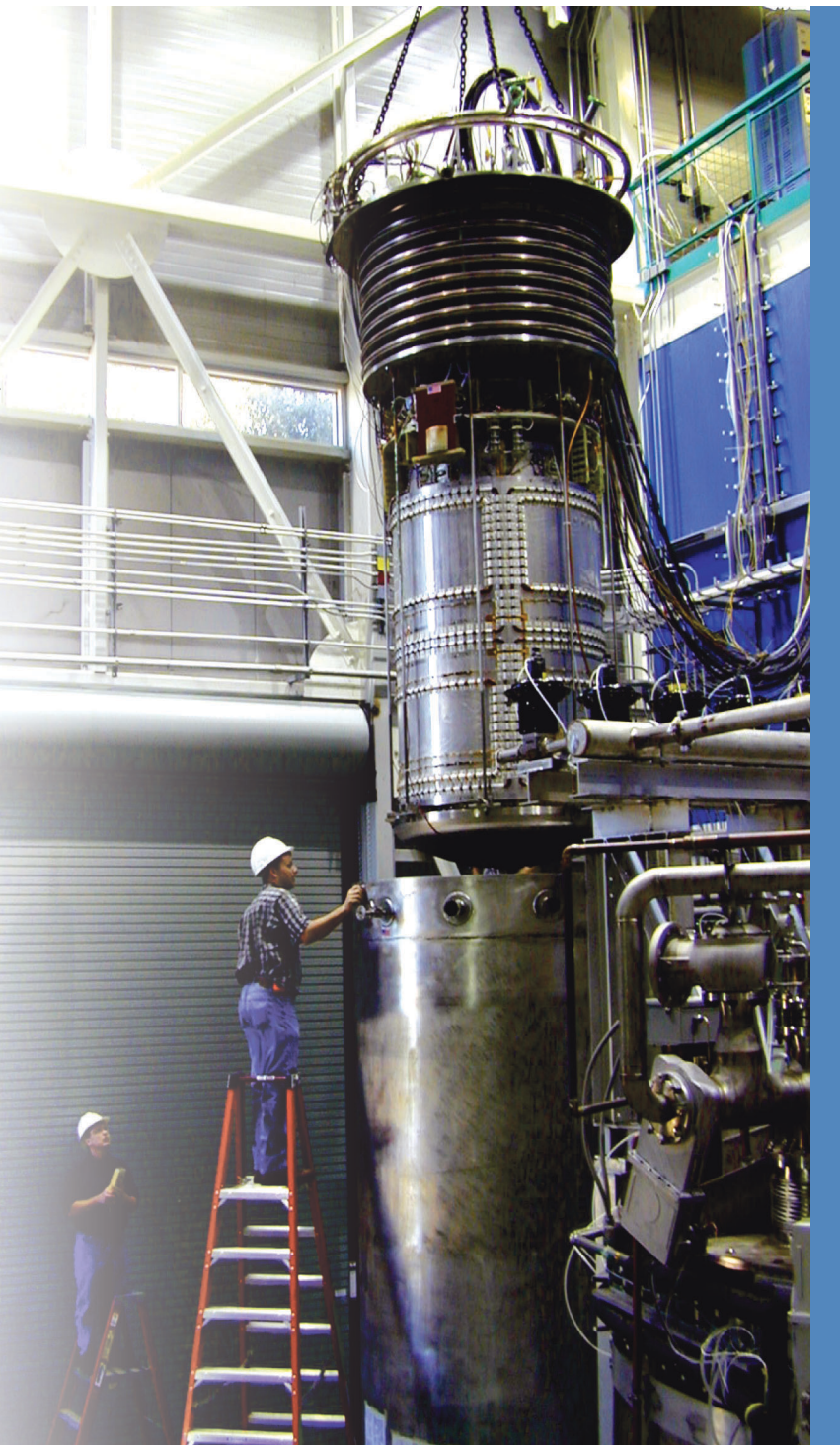
Figure 1. The magnet assembly is inserted in the bucket cryostat on October 26, 2001, in preparation for the initial bucket test.
