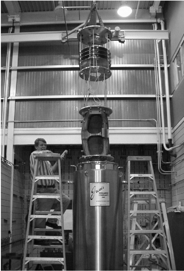
Figure 4. A coil /bobbin assembly is installed in a dewer at the NHMFL for high field testing.
