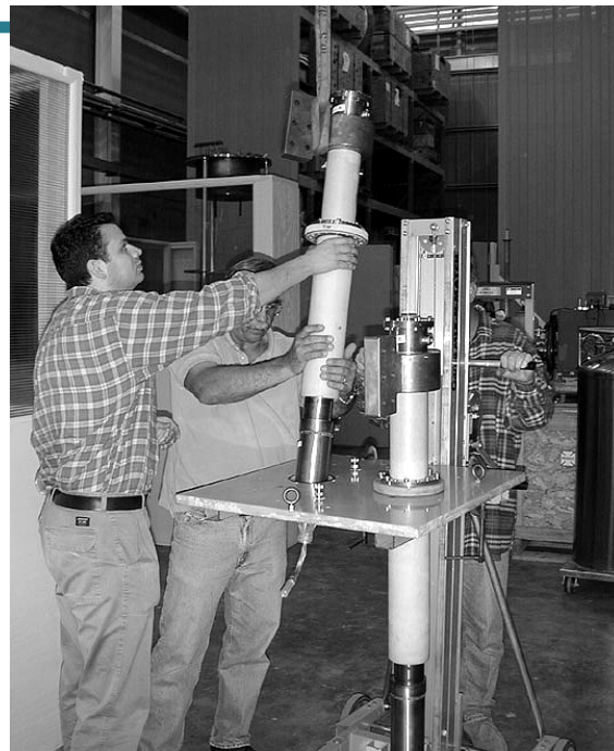
Figure 1. EURUS' Richard Hodges and NHMFL's Don Richardson and George Miller prepare the 13 kA leads for preliminary testing at NHMFL.
