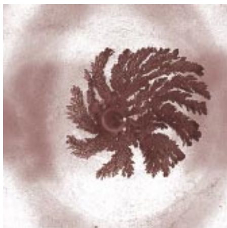
Figure 3. Two dimensional fractal copper electrodeposits obtained in zero field and in magnetic fields applied perpendicular ( \theta = 0, 180 ) or parallel ( \theta = 90 ) to the plane of the cell. a) B = 0\text{ T} b) B = 0.4\text{ T}, \theta = 0 c) B = 0.8\text{ T}, \theta = 180 d) B = 1\text{ T}, \theta = 90 .
