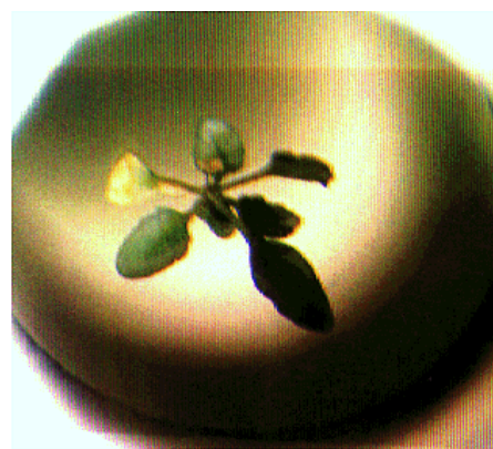
Figure 1. A magnetically levitated arabidopsis plant levitation in B = 14.4 T and B\nabla B = 1708 T 2 m -1 . The view is looking down the bore of the Keck magnet, and the scale is set by the diameter of the bore which is 52 mm.
