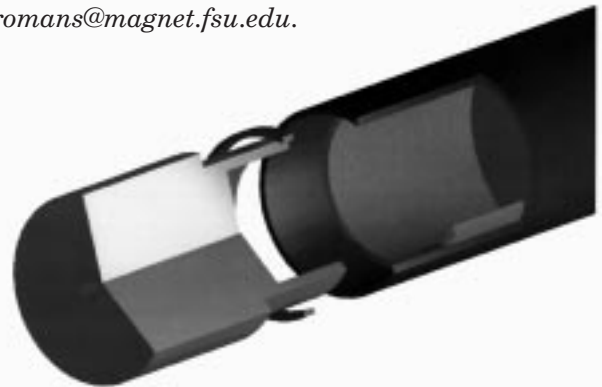
Figure 2. Rendered drawing of improved termination design for SL Series™ power leads (original drawing by NHMFL magnet designer Steve Kenney).
