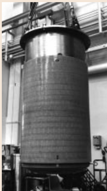
Figure 1. Five tons of assembled magnet swing free on their way to placement inside the liquid nitrogen dewar. Cool-down and electrical tests are next, followed by test pulses up to 60 T in early summer.
