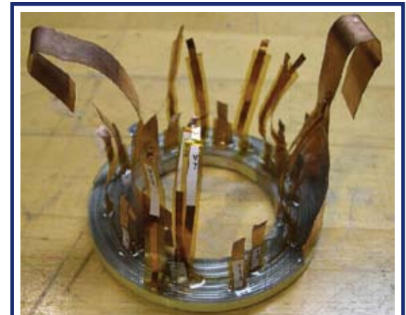
Figure 1. Epoxy impregnated pancake coil made of YBCO coated conductor. The coil is heavily instrumented for upcoming stability testing.
