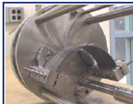
Figure 1. A pure bending device is shown in the figure. The superconducting strand is mounted on a support beam and a groove is placed on the neutral axis of the beam to produce pure bending effect on the strand.
