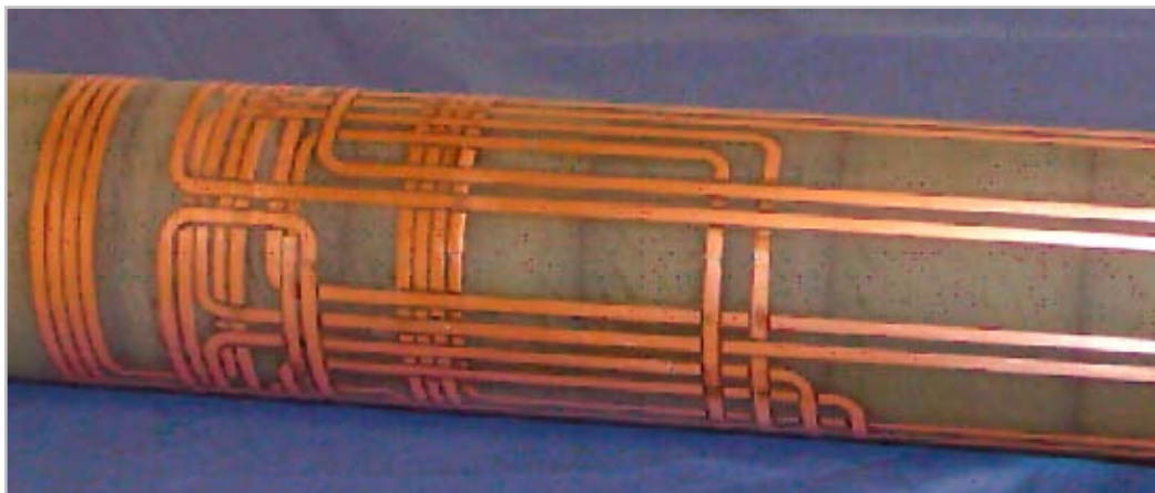
Figure 3. The water-cooled resistive shim set built for the Keck resistive magnet.
