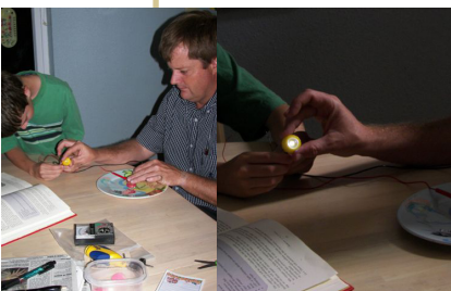
Depicted is an experiment where a kitchen battery powers a light emitting diode (LED). The Parkers found that an incandescent light bulb would not light, but that an LED would.
