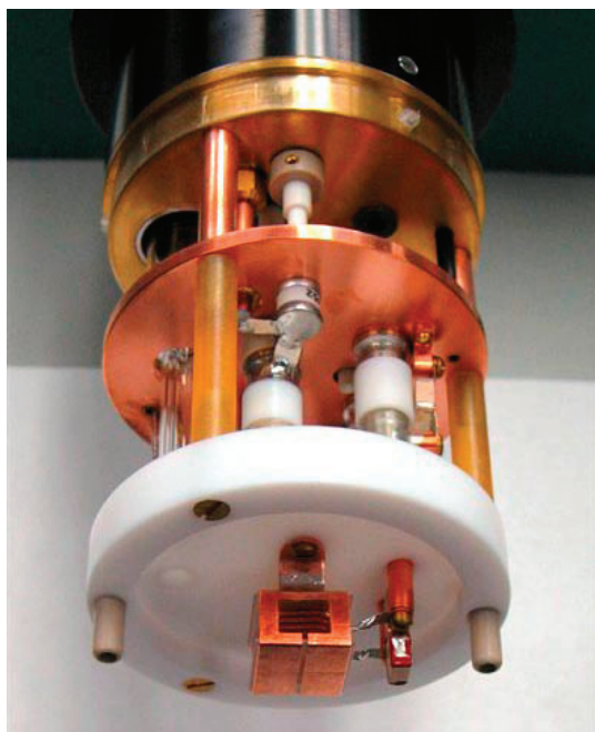
Figure 17. The 900 MHz low electric field probe that minimizes the electric field in the sample volume thereby minimizing the sample heating.
