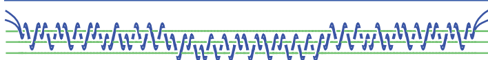
Figure 1. A braid that carries out a controlled-NOT gate between two qubits encoded using triplets of quasiparticles. A NOT operation is performed on the target (green) qubit if, and only if, the control (blue) qubit is in the state |1\rangle .
