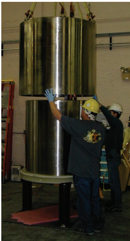
Figure 4. Coil number 7 being installed on the 100 T MS magnet.
