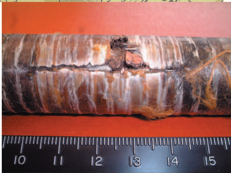
Figure 2. Layer 1 mid-plane fault illustrating short between turns.
