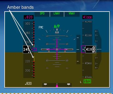
Pilot Tip The minimum maneuver speed indication does not guarantee the ability to maintain level flight at that speed.
