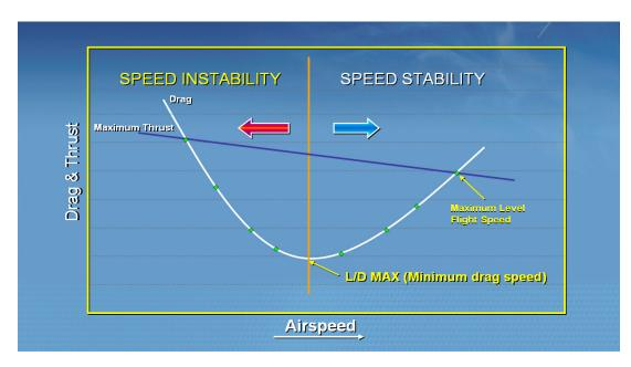
Figure 1. Airspeed versus drag in level flight
