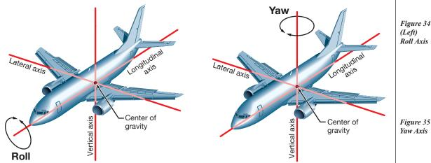
Figure 34 (Left) Roll Axis
