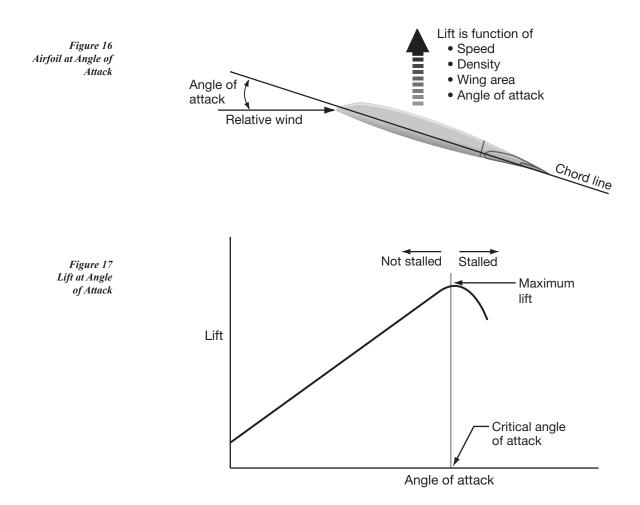
Instead of increasing with an increase in angle of attack, it decreases. At this critical angle of attack, the air moving over the upper surface can no longer remain attached to the surface, the flow breaks down, and the surface is considered stalled.
