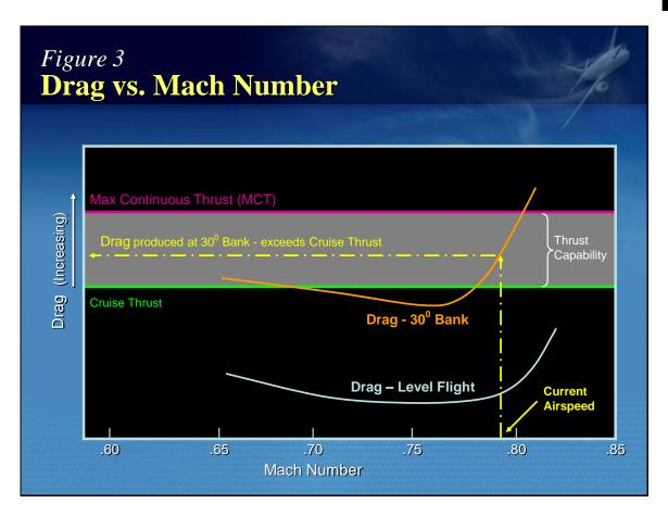
• Figure 3 shows that for normal cruise speeds there is excess thrust available at this fixed weight and altitude. When trying to turn at 30 degrees of bank the drag exceeds the normal maximum cruise thrust limit. If the pilot selects maximum continuous thrust then there is enough thrust to maintain the bank angle in the same situation.
