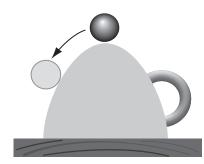
**Unstable** When ball is displaced, it accelerates from its original position.
