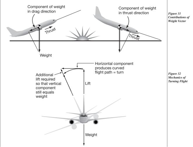
the only way to generate a sideways-pointing force, but it is the typical method.
