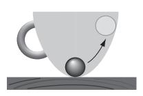
**Stable** When ball is displaced, it returns to its original position.
