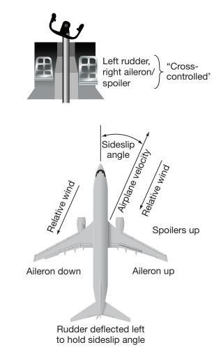
Figure 25 Angle of Sideslip With the exception of crosswind landing considerations requiring pilot-commanded sideslip, commercial transport airplanes are typically flown at or very near zero sideslip. This usually results in the lowest cruise drag and is most comfortable for passengers, as the sideways forces are minimized.
