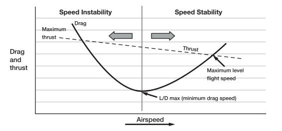
Figure 39 Airspeed Versus Drag in Level Flight
