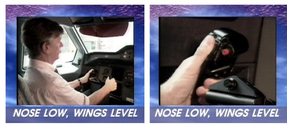
Apply noseup elevator
