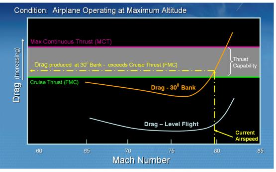
Figure 3. Drag reduced by bank versus available thrust
