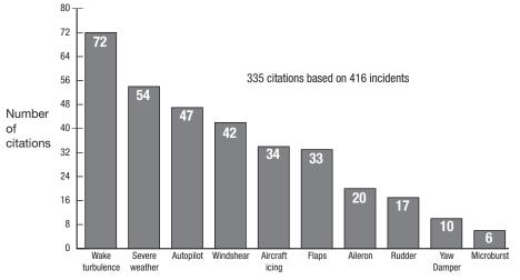
Figure 2 Multiengine Turbojet Loss-of-Control Incidents, January 1996 to August 2002, ASRS
