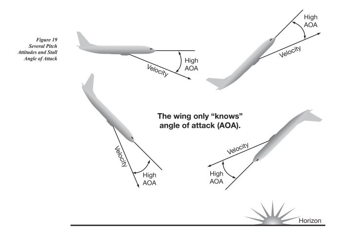
should not expect the airplane to remain unstalled just because the indicated airspeed is higher than AFM chart speeds, because the conditions may be different.
