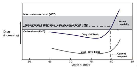
Figure 41 Drag Induced by Bank Versus Available Thrust
