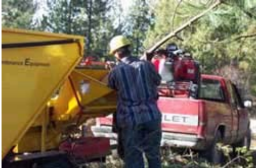
Figure 48. Chipping slash with a CT-24 chipper. Slaughterhouse Gulch, Boise National Foest, 2001.
