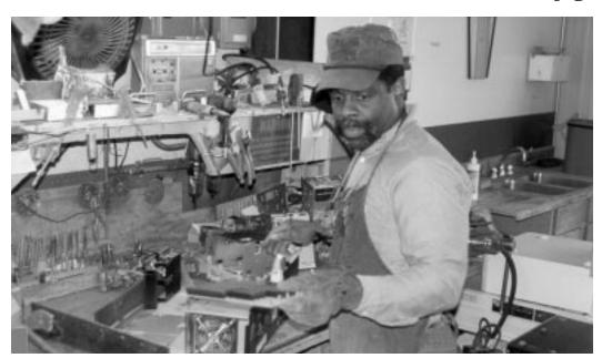
An employee from Morningside, a community rehabilitation program, removes precious metals components of a disassembled computer at Fort Lewis Army Base in Tacoma, Washington. The operation to recover metals is a JWOD contract.
