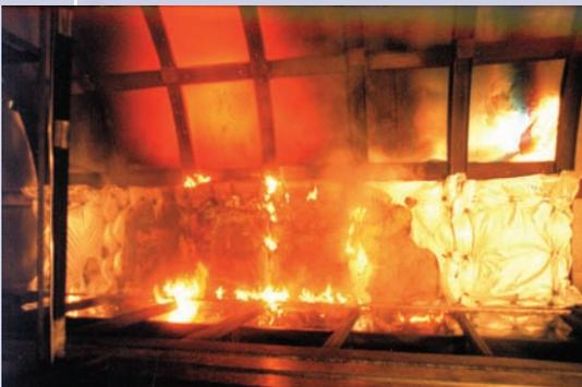
strips of tape. The advisory circular also requires testing for structural damping materials. For example, although small aluminum sheets bonded directly to the airplane skin are not considered insulation, materials that include a layer of foam or other material sandwiched between the skin and thin aluminum sheets should be tested.
