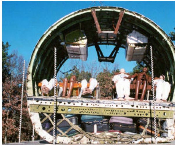
Figure 2. B737 Fuselage Section with Overhead Stowage Bins
