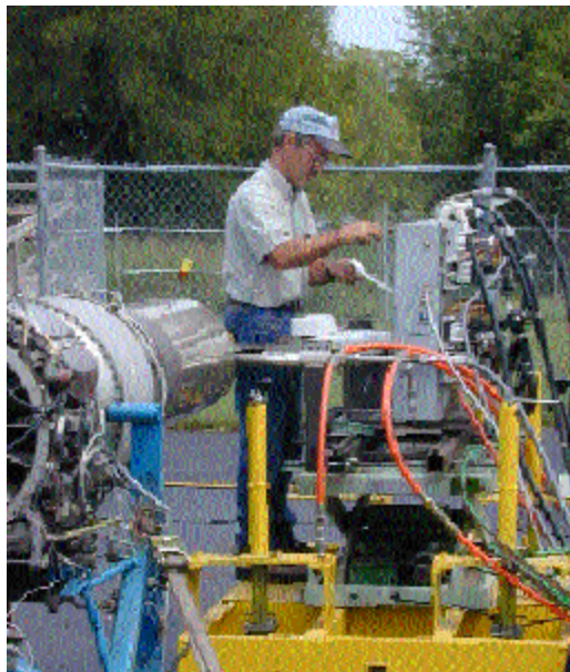
Readying equipment for hazardous air pollutant sampling of a jet engine
