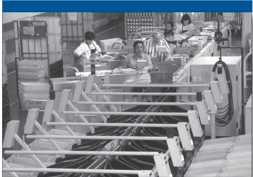
To increase efficiency and reduce the cost of processing flats mail by more than $7 million annually, the Office of Audit recommended using the Upgraded Flats Sorting Machine 1000's automated feeder in the optical character reader mode rather than keying addresses.
