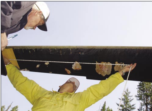
Investigators measure scrape marks on the helicopter’s main rotor blade, after emergency landing.
