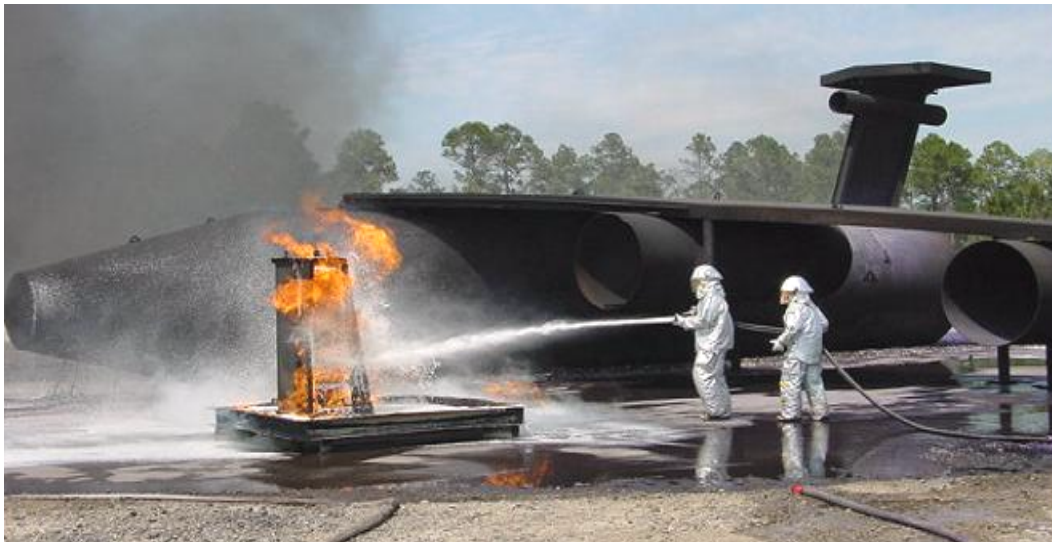
FIGURE 4. CASCADING FUEL FIRE TEST ARTICLE
