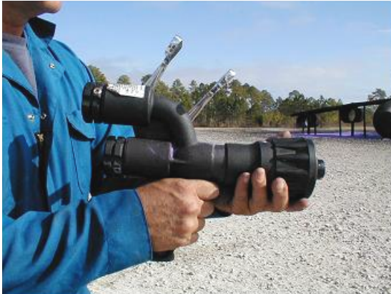
FIGURE 2. DUAL-AGENT, VARIABLE-STREAM NOZZLE
