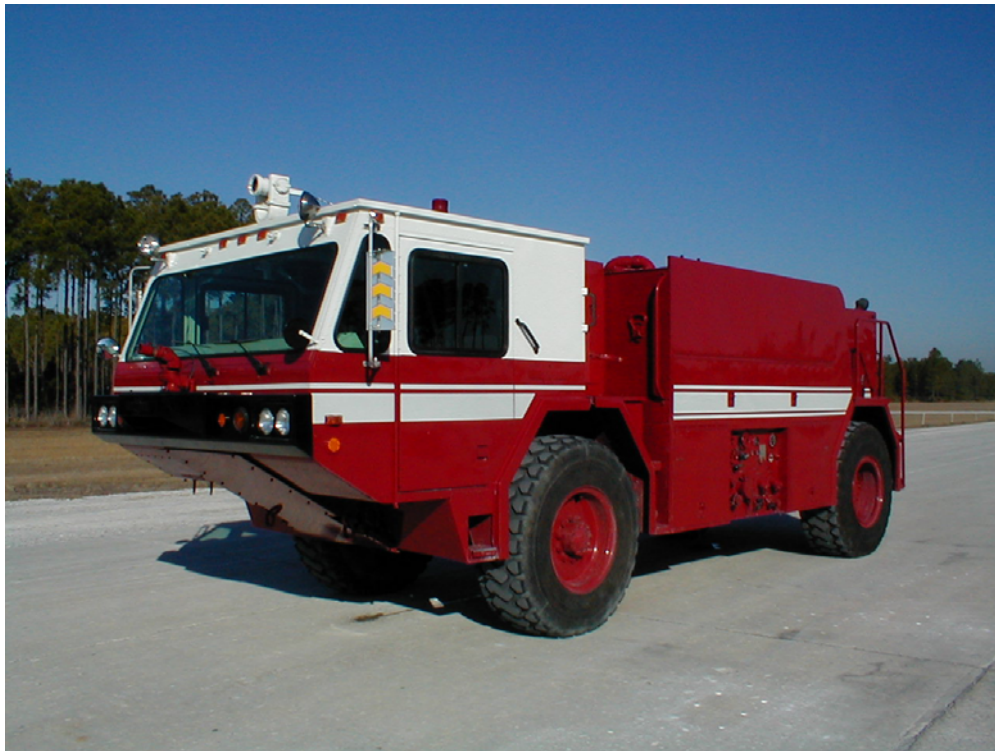
FIGURE 8. UNITED STATES AIR FORCE P-19 CRASH TRUCK
