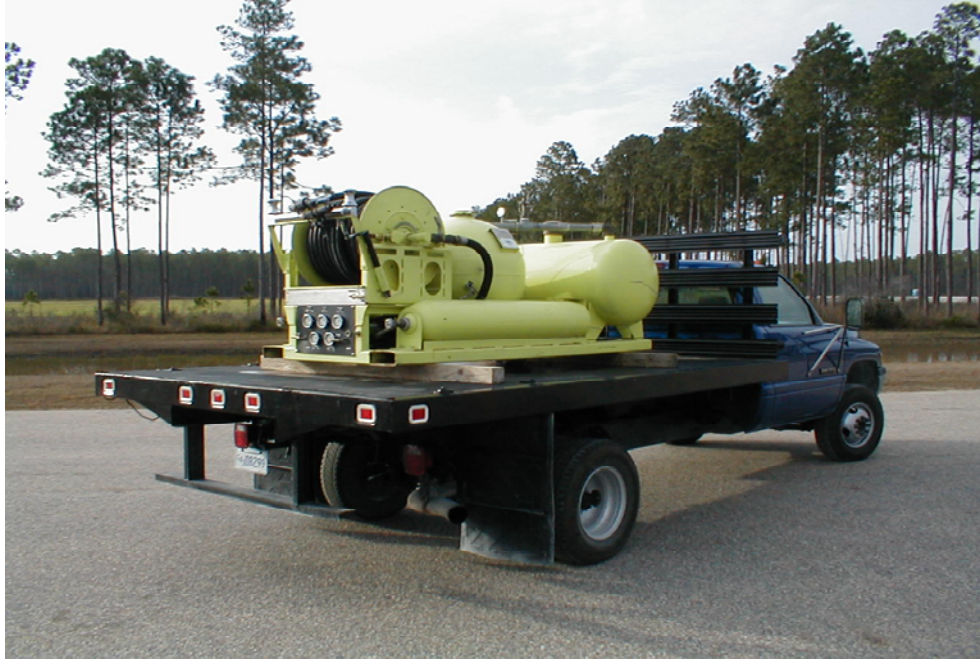
FIGURE 1. SMALL AIRPORT FIREFIGHTING SYSTEM MOUNTED ON TEST SUPPORT VEHICLE
