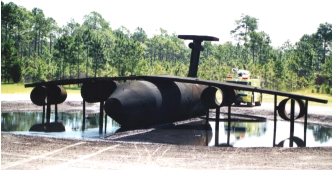
FIGURE 6. LARGE-SCALE FIRE TEST SETUP
