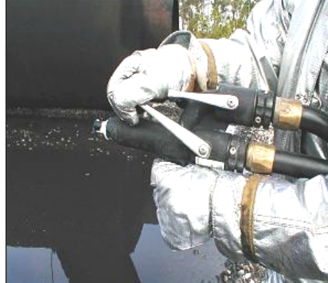
FIGURE 3. DUAL-AGENT, COMPRESSED AIR FOAM NOZZLE
