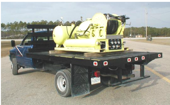
FIGURE 9a. STAKE BODY TRUCK WITH SAFS
