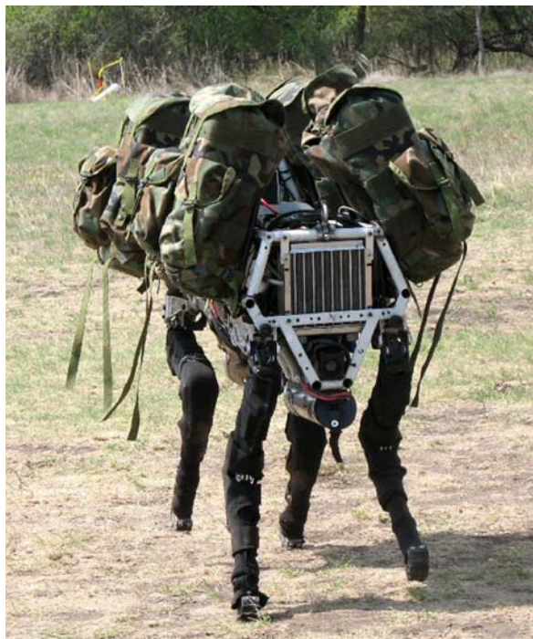
Figure 35: Bio-inspired “Big Dog” quadruped robot is being developed as a “mule” that can traverse difficult terrain.
