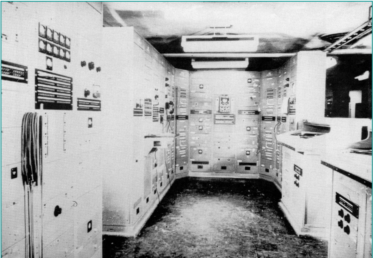
Fig. 1. A view of SIGSALY through the rear doors of a tractor trailer. The first real-time secure voice system, circa 1944
