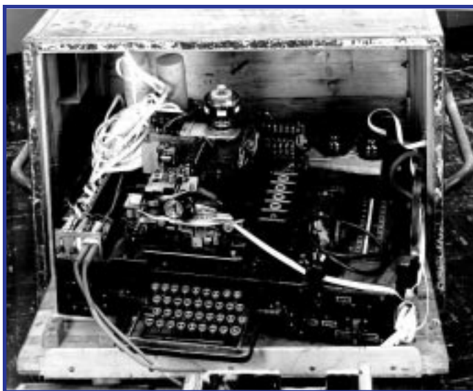
Fig. 8. TUNNY teletype base, in safe
