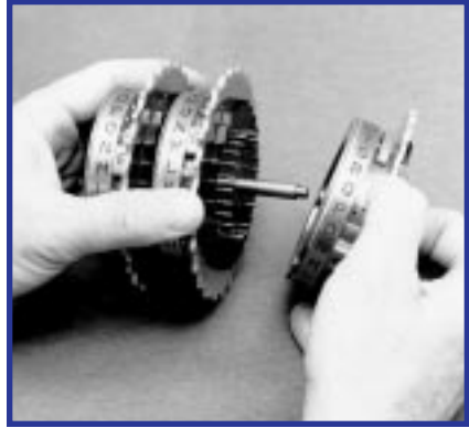
Fig. 4. Assembling the rotor set
