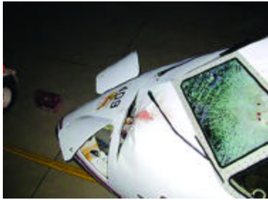
Bird strike damage
