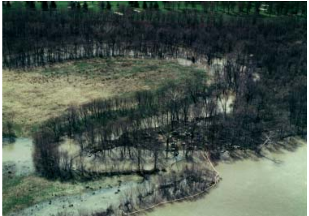
Booms used to control oil entering the Potomac at the mouth of Sugarland Run. National Park Service photo.
