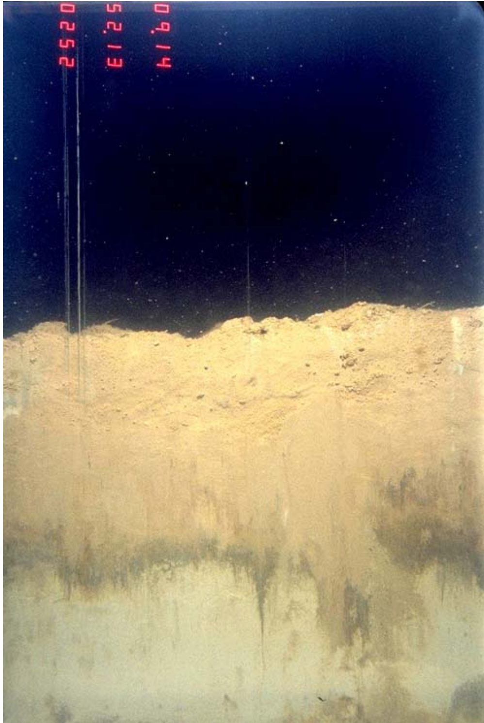
Plate 12. Sediment profile image from the near-field site at Garden Banks Block 516 during Cruise 2B. The upper few millimeters of the sediment consist of sand-sized grain aggregates; four layers of oxidized and reduced sediments are visible. Station NF1-6B. Image width is 15 cm.
