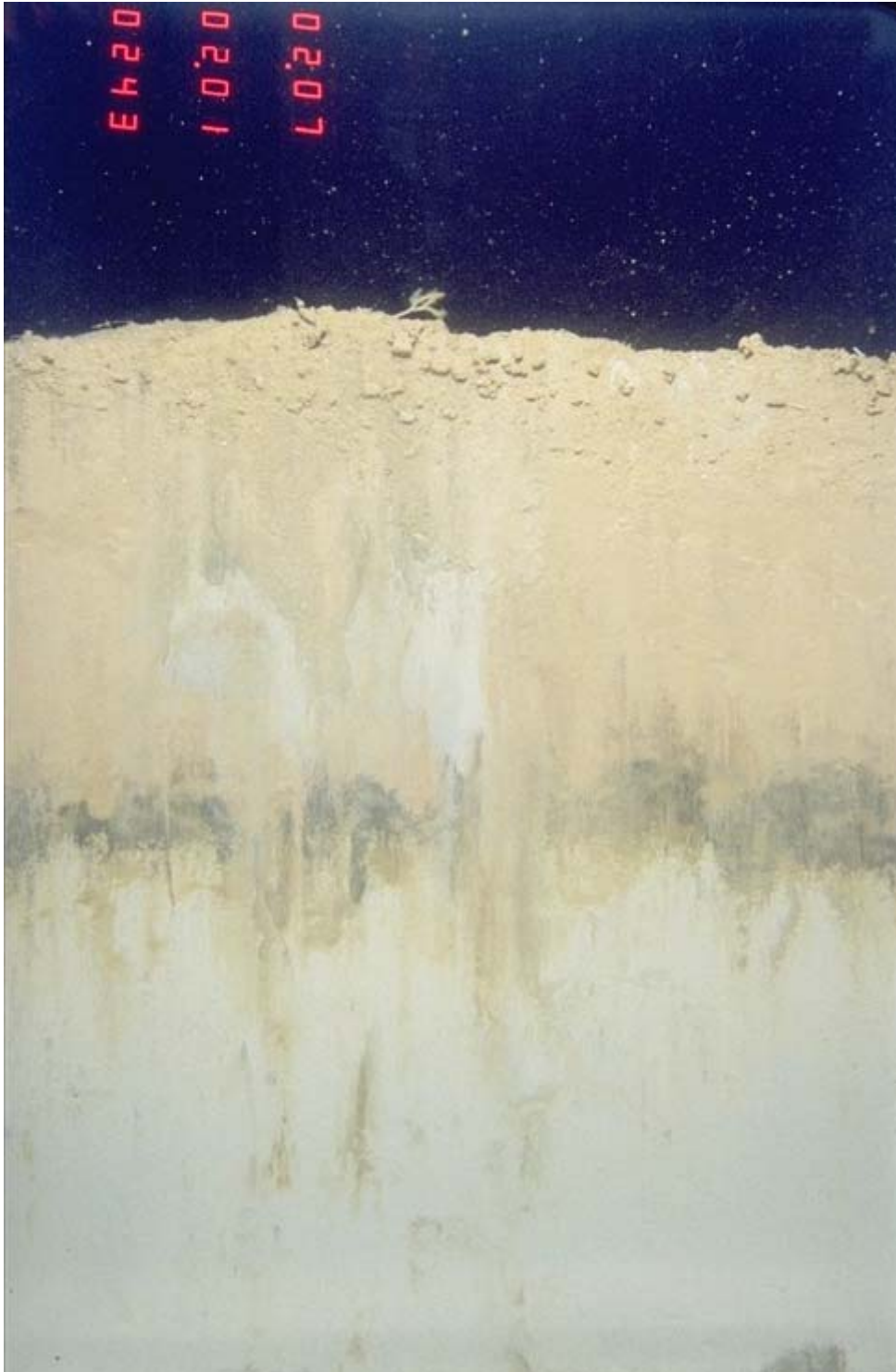
Plate 7. Sediment profile image from a far-field site at Garden Banks Block 516 during Cruise 1B showing pink to tan mottled surface sediments underlain by a thin layer of sulfidic gray to black sediment, which in turn, overlies a homogeneous light gray layer. Station FF6-S3.13. Image width is 15 cm.
