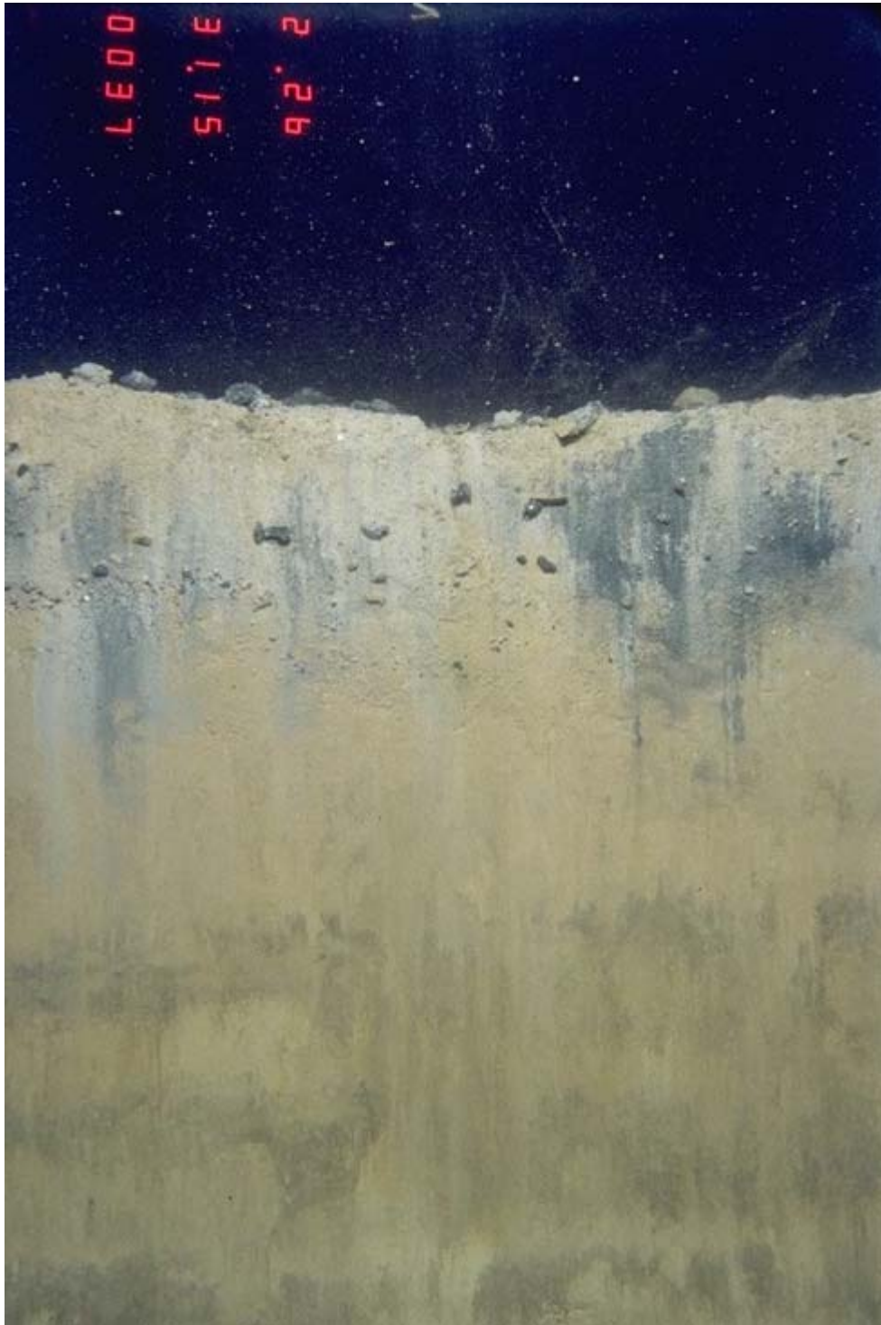
Plate 1. Sediment profile image from the near-field site at Garden Banks Block 516 during Cruise 1B showing a granular surface layer of pink to reddish-tan sediment underlain by a dark gray to black sulfidic layer. Station NFS-1.19. Image width is 15 cm.
