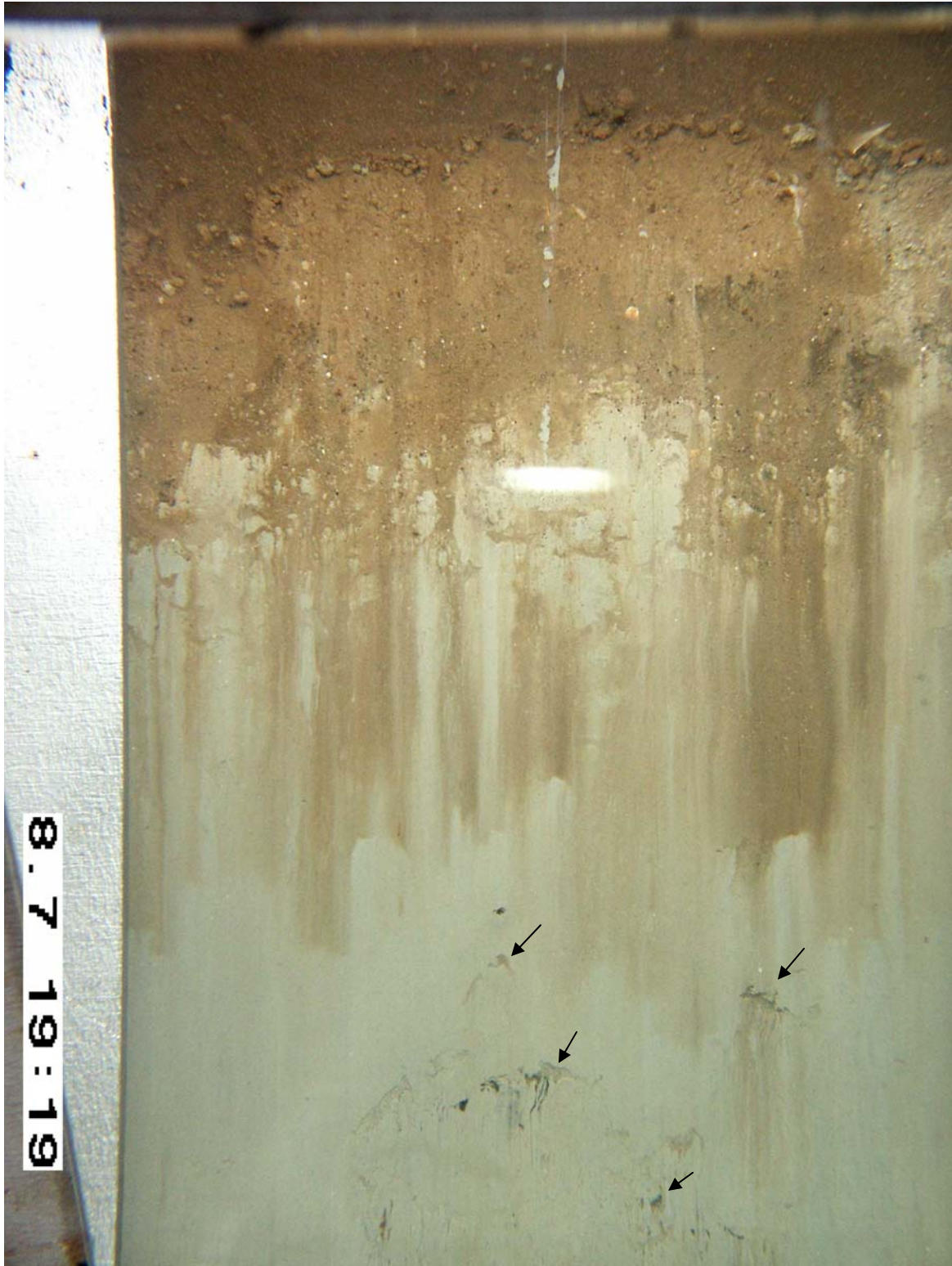
Plate 21. Sediment profile image from the near-field site at Viosca Knoll Block 916 during post-drilling Cruise 3B showing numerous infaunal feeding voids (arrows). Station NF1-37 (1919). Image width is 15.2 cm.
