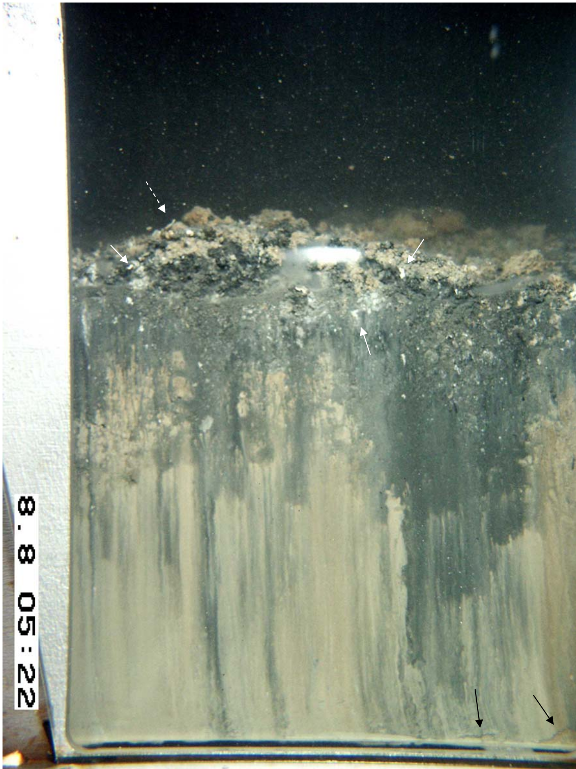
Plate 30. Sediment profile image from the near-field site at Viosca Knoll Block 916 during post-drilling Cruise 3B showing sulfidic areas within the layer of red to reddish-gray sediment. Station NF3-34 (0522). Thin strands of a small disturbed bacterial mat are visible in the upper layer (white arrows). A region of chaotic fabric is still present between the upper layer and the homogeneous gray clay. A recumbent tube is present on the surface (white dashed arrow). Feeding voids are visible at depth (black arrows). Image width is 15.2 cm.
