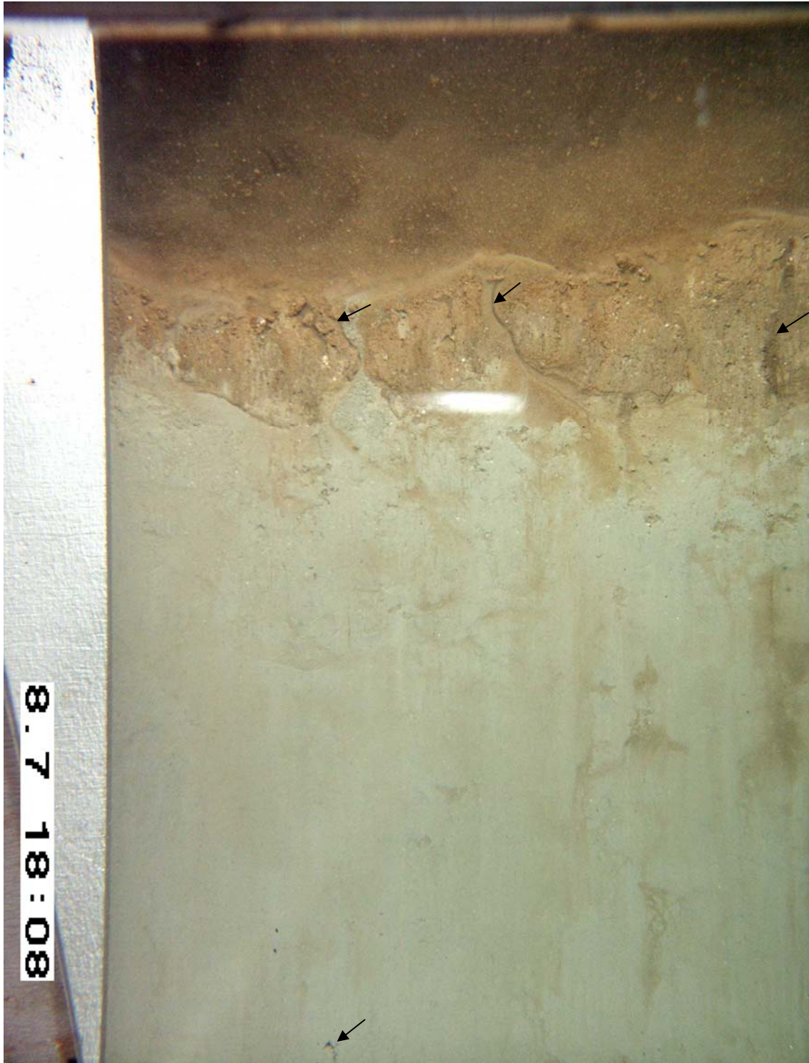
Plate 20. Sediment profile image taken in the near-field site at Viosca Knoll Block 916 during post-drilling Cruise 3B showing a layer of red to reddish-gray sediment over a region of chaotic fabric, which in turn, overlays a homogeneous gray clay. Station NF1-01 (1808). The surface is erosional, and no Stage I tubes are visible. Dewatering channels are present (3 arrows near surface) in the uncompacted surface region. A tiny feeding void (arrow) is present at 18-cm depth. Image width is 15.2 cm.
