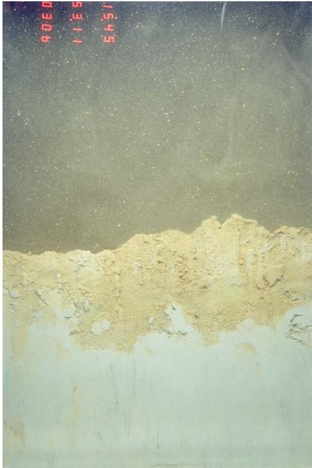
Plate 11. Sediment profile image typical of the far-field sites sampled during pre-drilling Cruise 1B at Viosca Knoll Block 916. Station FF6-S3.18. Image width is 15 cm.
