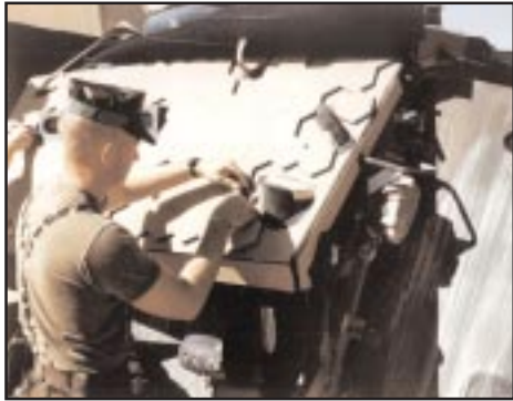
■ A marine adds DARPA/DSO ceramic armor appliques to a light armored vehicle.
