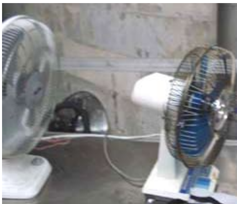
Figure 1: Fans used for cooling can cause lead paint particles to be airborne and inhaled.
