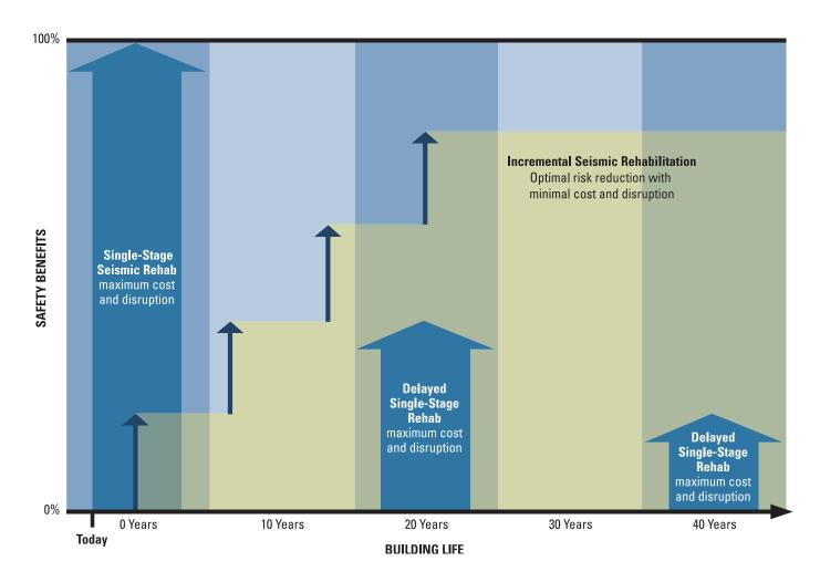
Incremental seismic rehabilitation affords great flexibility in the sequence and timing of actions when the following precautions are kept in mind:
