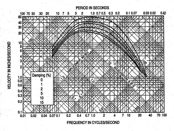
Figure 1: Seismic Design Response Spectra for Electrical Substation Equipment (from City of Los Angeles, 1988).
