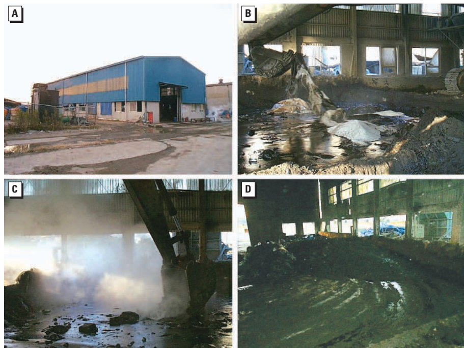
Figure 1. Process of unslaked lime solidification reaction. (A) Reaction is performed in a warehouse with the windows removed. (B) For each reaction, 100–250 drums of liquid wastes and 7–12 tons of unslaked lime are loaded in a constant ratio with liquid wastes. (C) As the wastes and unslaked lime are mixed, thick noxious vapors rise during the heat reaction and escape through the open windows; the full reaction takes > 12 hr with emission of huge amounts of noxious gases and vapors. (D) Final stage of the process after 10 hr of thermochemical reaction.
