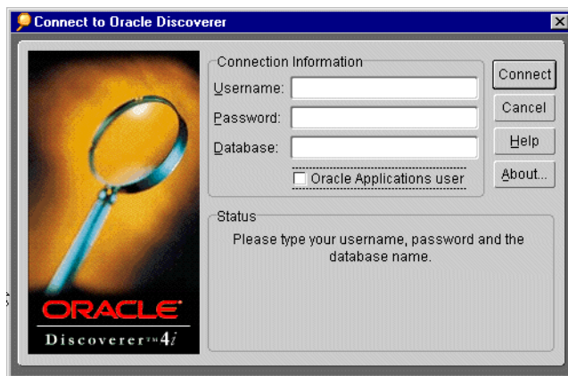
Figure 5-4 An Oracle Discoverer Connect dialog for Applications Users or standard EUL Users
