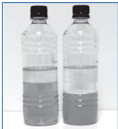
Figure 2.5. Bottles containing oil and water can simulate people with different body types.
