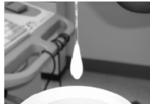
Figure 3 A 3-mm cryoprobe that has been inserted into water and activated for 30 seconds. This image shows the profile of the image.
