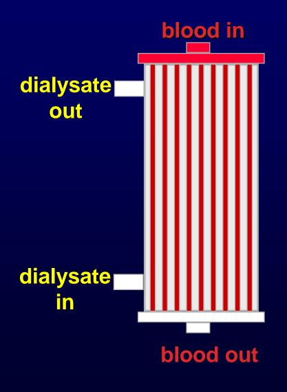
Cross Section hollow fiber membrane
