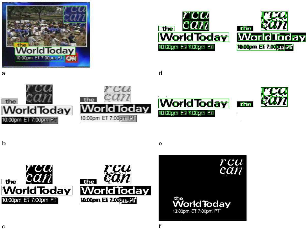
Fig. 4a–f. Steps of the binarization algorithm: a video frame marked with localized text boxes; b preprocessing is applied on each text box, and the inverse of each is obtained; c logical level thresholding is applied to both polarities; d connected component analysis is performed and heuristics remove non-character components; e correct polarity for each text region is chosen; f final binarization result
