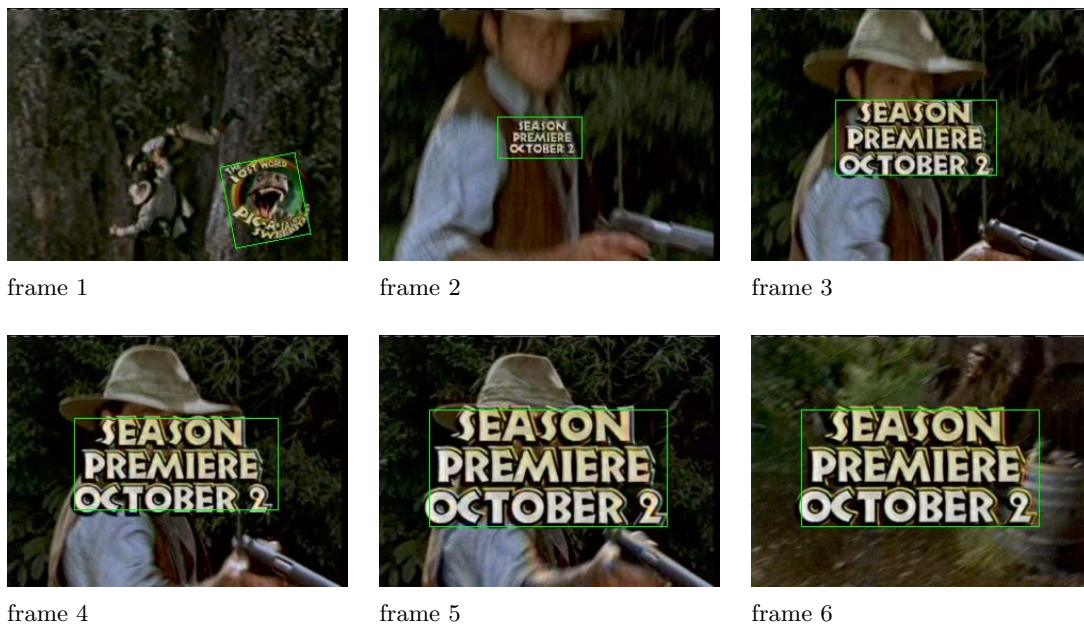
Fig. 14. Sample results of combined text detection and tracking on growing text against an unconstrained background
