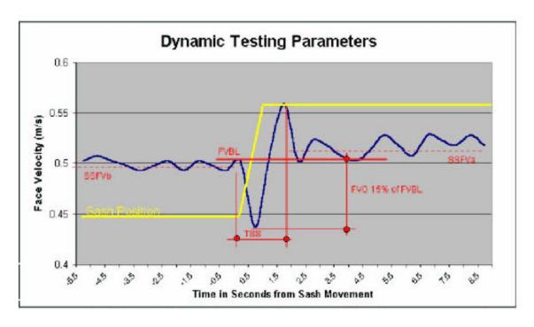
q) Turbulence Intensity (TI expressed in m/s): Calculated root mean square of the fluctuating face velocity determined using FVm, calculated as follows:
