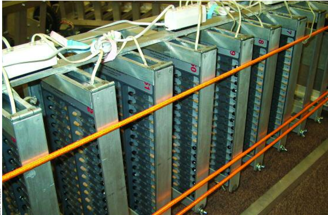
▲ This contraption turns on its side like a carnival ride to keep the flies inside each vial awake.
