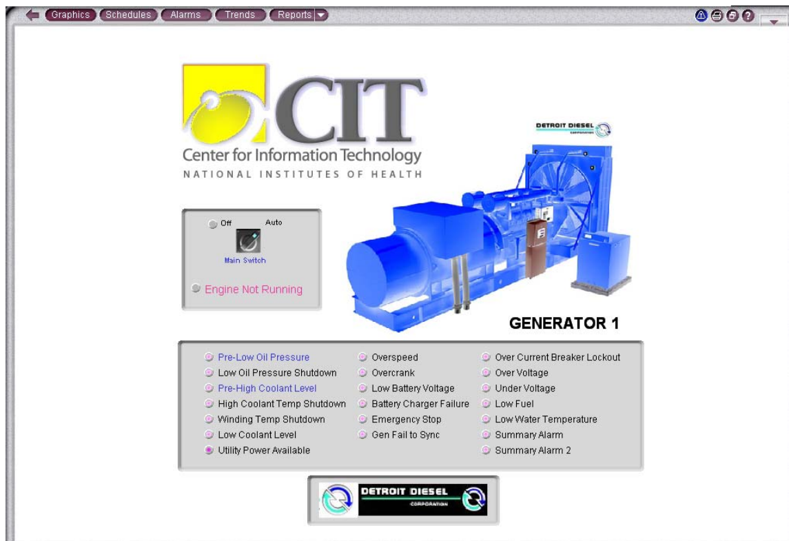
(Illustration 3) Generator 1: WebCTRL tracks 21 conditions for each generator, including oil pressure, coolant level, battery voltage, fuel level, and water temperature.
