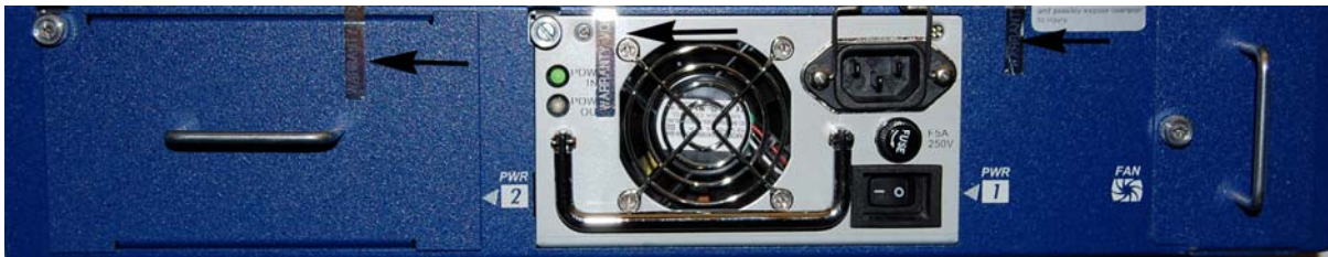
Fig. 2: Rear of NetScreen-500, with location of temper evident seals
