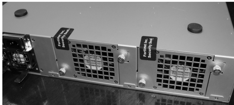
Figure 5: FortiGate-1000A and 3600 fan assembly seals
