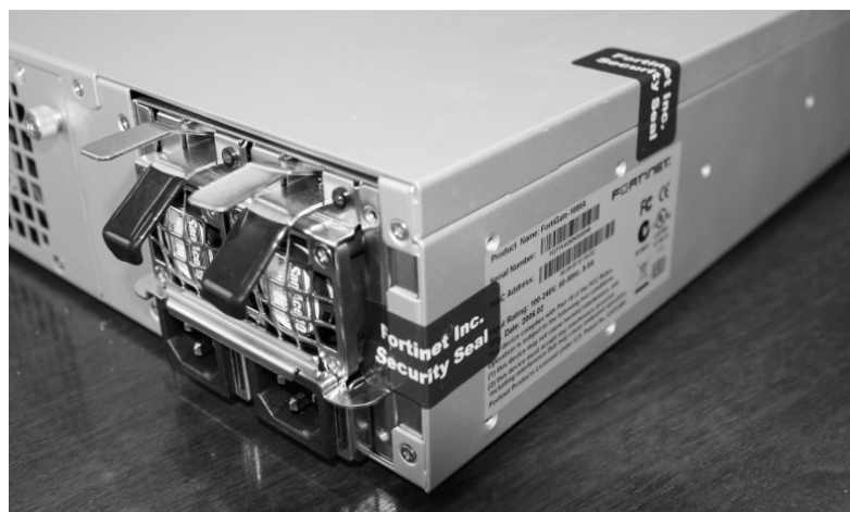
Figure 4: FortiGate-1000A and 3600 external enclosure and power supply seals
