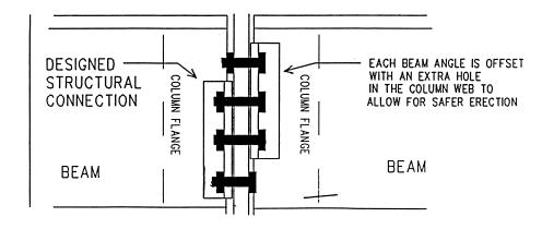
Staggered connections are connection material on a structural member in which all of the bolt holes in the common member web are not shared by the two incoming members in the final connection. The extra hole in the column web allows the erector to maintain at least a one bolt connection at all times while making the double connection.
